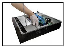
Figure 1-24 Fix the HDD
