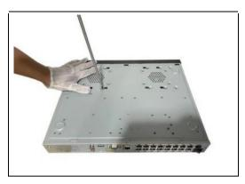
Figure 1-19 Fix the HDD
