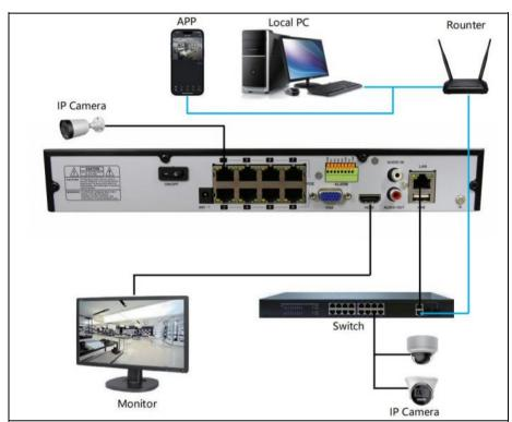
Figure 1-30 Device connection
