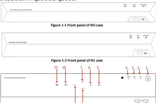
Figure 1-3 Front panel of W1 case
