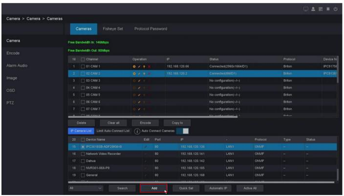
4. Check the status of the camera, 'Connected' means connected, 'Connecting' means connecting, 'identifying error' means the password is incorrect, except 'Connected', all others need to check the connection information to ensure that the camera can be connected normally.
