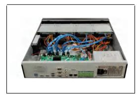
Figure 1-23 Connect the power and data cables
