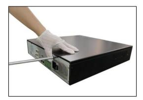
Figure 1-25 Install the cover and screws
